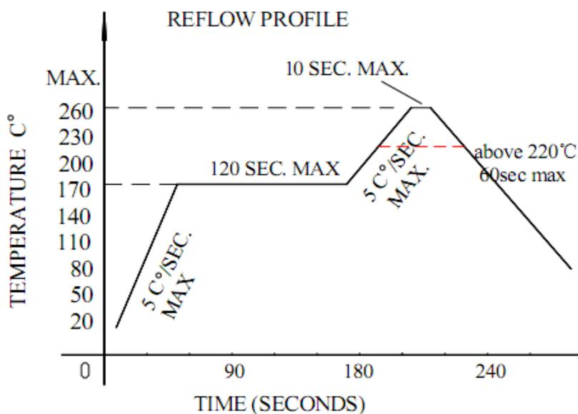
1. Reflow soldering should not be done more than two times
